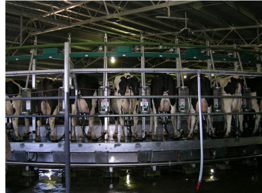
80 stand rotary, computerized milking parlor. (2009) 122
